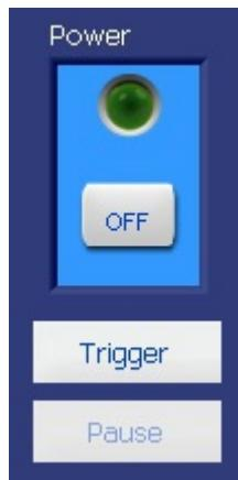
**Power:** Indicates the output state of the power supply.
