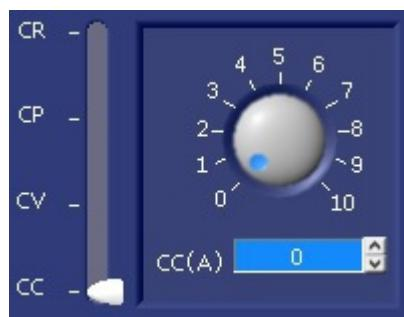
This part provides three ways to set the parameters. Select the desired operation mode (CR, CP, CV or CC) first, then
